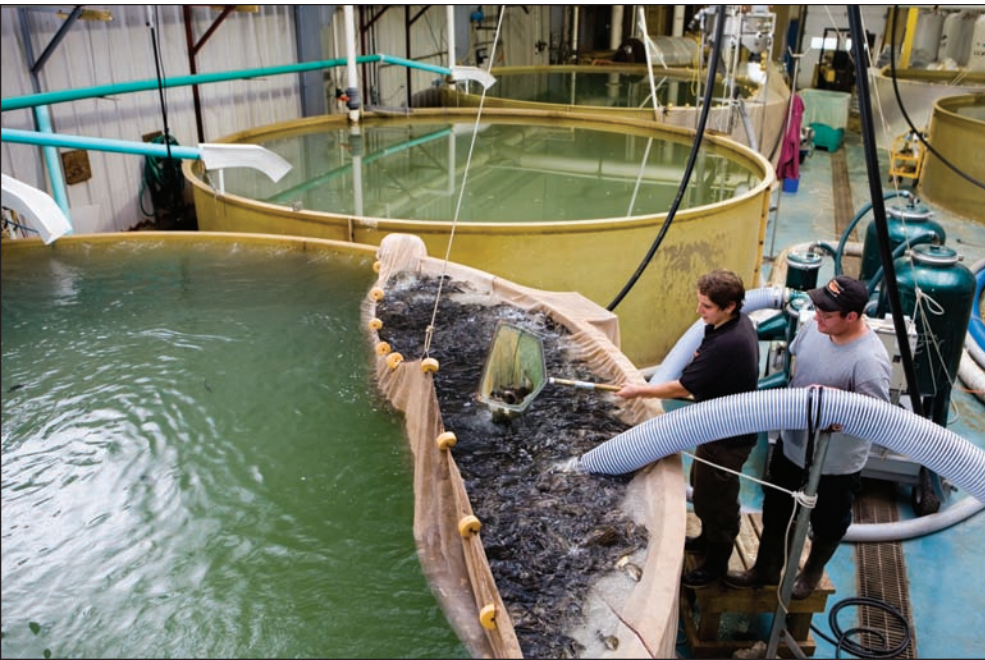
THE MULTIPLICATION FACTS Aquaculture technicians at the Australis facility in Turners Falls vacuum juvenile fish from a nursery tank to electronically sort and count them.
